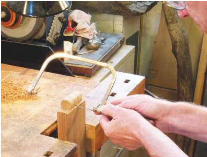
▲ Pic.11 Severing the middle knuckle
